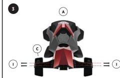
Attach Armrests: Attach them to the seat frame using screws (provided). Make sure they are securely fastened.
