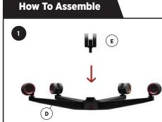
Attach Casters to Base: Simply insert the stem of each caster into the holes in the base and push until they snap into place. Make sure they are securely attached.
