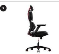
Attach Seat to Base: Align the mounting holes on the bottom of the seat with the holes on the chair base. Push until they snap into place.
