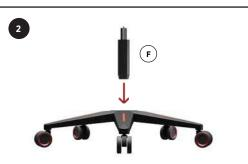
Attach Gas Lift Cylinder: The gas lift cylinder is responsible for adjusting the height of the chair. Slide the gas lift cylinder into the center hole of the chair base. It should fit snugly.
